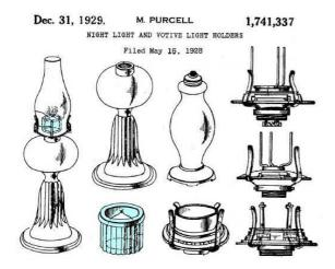
In this simplified and colorized version of the patent drawing, you can see how the candle cup was to be used. They details of the burners simply illustrate the "adapters" that are to be used to support the candle cup.
